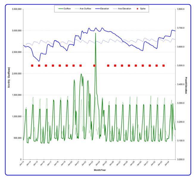
2 3 4 5 FIGURE 7 Comparison of Monthly Outflow and End-of-Month Elevation of Trace 14 and the All-Trace Average for Alternative F
