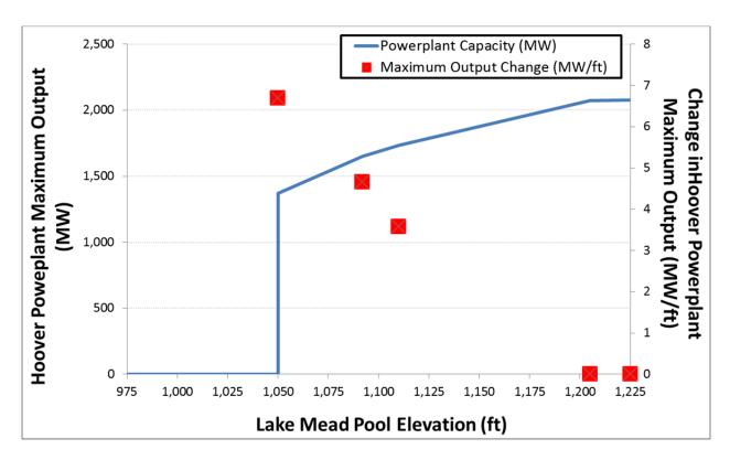
FIGURE K.5-12 Hoover Powerplant Maximum Physical Output as a Function of Lake Mead Pool
