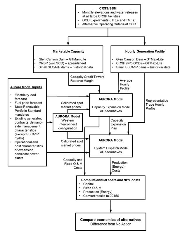
FIGURE K.1-5 Flow Diagram of the Power Systems Methodology Used in the LTEMP DEIS
