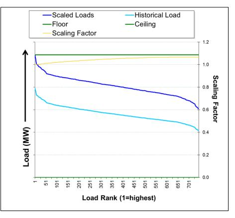
FIGURE K.1-9 Example of the Load Scaling Algorithm LDC
