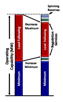
FIGURE K.1-22 Reductions in Operating Range when Providing Ancillary Services
