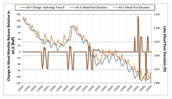
FIGURE K.5-10 Alternative F Changes in Monthly Hoover Powerplant Turbine Water Releases under Hydrology Trace 8
