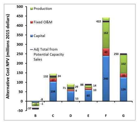
FIGURE K.1-52 Cost Difference of Alternatives Compared to Alternative A at 90% Exceedance Level and 3.375% Discount Rate Assuming Average Hydropower Conditions
