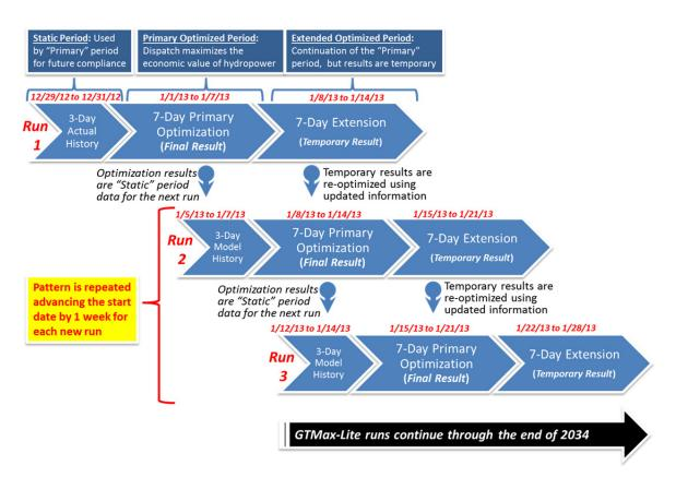
FIGURE K.1-8 Illustration of Temporal Modeling Method Used in the GTMax-Lite Five
