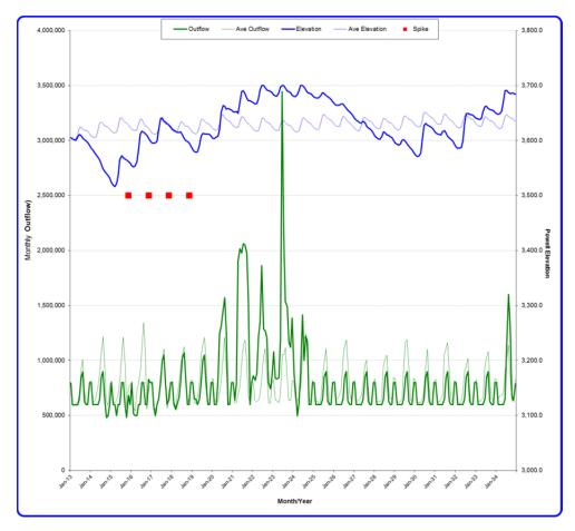
FIGURE 6 Comparison of Monthly Outflow and End-of-Month Elevation of Trace 14 and the All-Trace Average for the No Action Alternative
