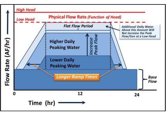
FIGURE K.1-24 Illustration of Ramping Time Increase as a Function of Increasing Water Volumes at Flaming Gorge Dam
