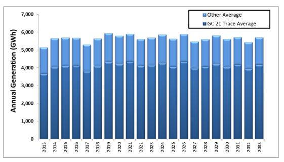
FIGURE K.1-34 Annual Average Hydropower Generation for the Glen Canyon Dam Powerplant and the Aggregate Generation for all other SLCA/IP Resources
