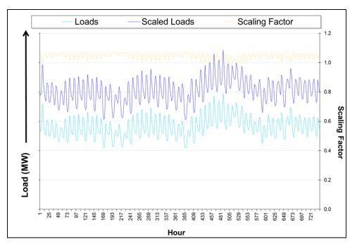
FIGURE K.1-10 Example of the Load Scaling Algorithm Chronological Hourly Loads
