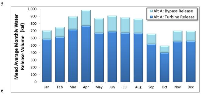
FIGURE K.5-6 Average Monthly Turbine and Bypass Water Releases
