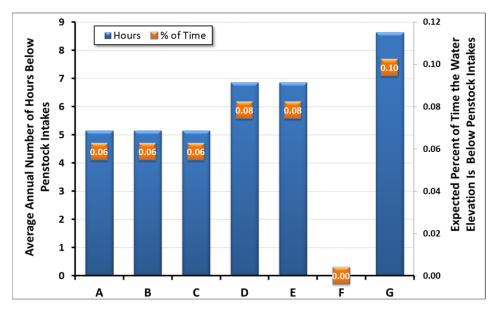
FIGURE K.1-43 Average Annual Number of Hours the Lake Powell Elevation Is below the Penstock Intake by Alternative for All 21 Hydrology Traces of Sediment Trace 2
