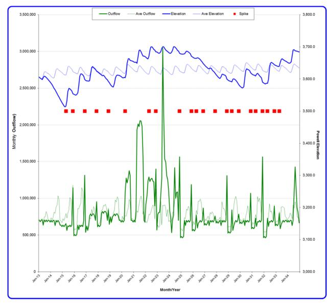
2 3 4 FIGURE 8 Comparison of Monthly Outflow and End-of-Month Elevation of Trace 14 and the All-Trace Average for Alternative G
